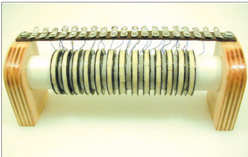
Assembled LF/VLF aerial-to-receiver matching tapped inductor coil
